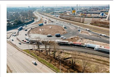
The R4WO project will transform the R4 West and East into primary roads in Ghent, Evergem, Zelzate and Wachtebeke. The project consists of the conversion of 18 intersections. In 2021, we started work on the first four of these intersections, which had been marked as 'quick wins'. The work consists of the construction of three bicycle tunnels on the R4 West and the transformation of the Euro-Silo intersection on the R4 East into a turbo roundabout.
