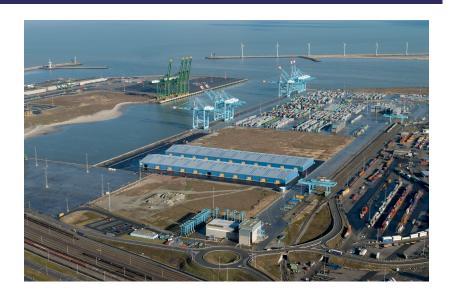
For MBZ nv (Port of Zeebrugge), Aswebo is surfacing the quay of the Albert II dock in Zeebrugge, with two new underlayers and a top layer of asphalt after the laying of the crane rails. Aswebo is also renovating the drainage system. The total area is 27,500 m². The site will be used by the companies Verbrugge and APM Terminals.
